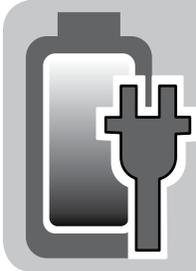
**IMPORTANT!** Before using the unit for the first time the battery needs to be charged for at least **8 to 12 hours** - no more than **20 hours**. Only an adult who has read and understands the safety warnings should handle, charge or recharge of the battery (see Maintenance).
