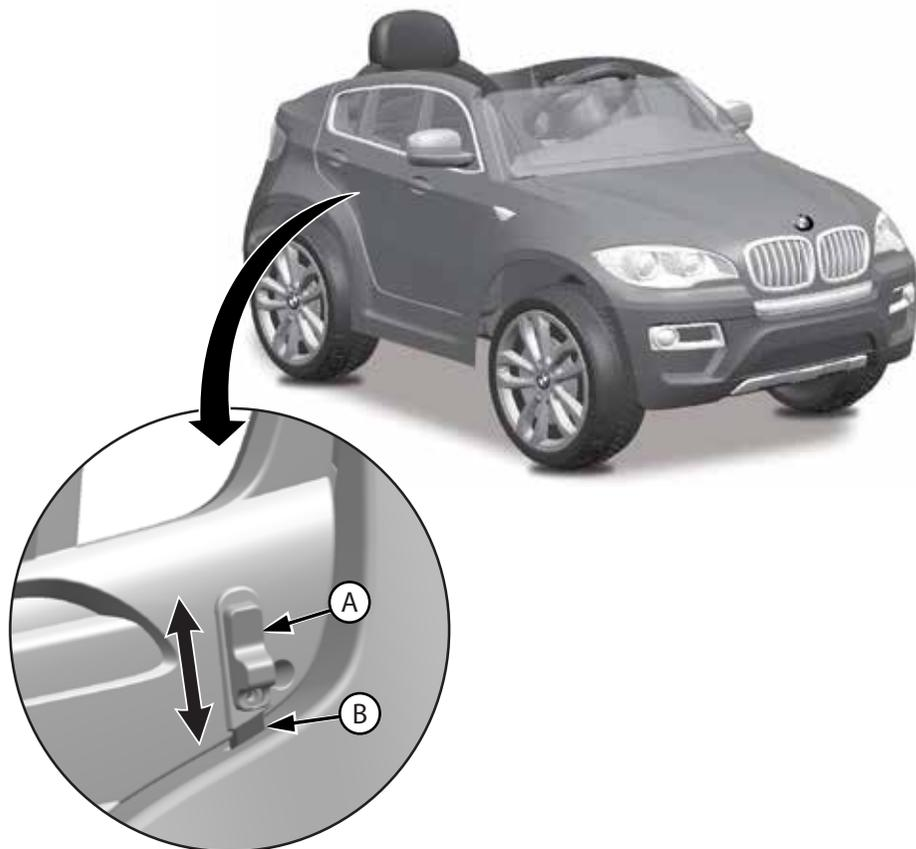
**This vehicle is equipped with Door Locks (A) on each door.**
