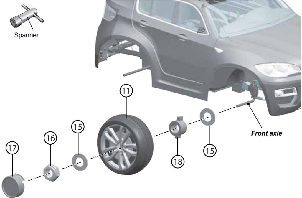
**NOTE: Begin by removing nuts and washers from axles.**
