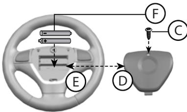
5. With a small screwdriver remove the **screw (C)** on the **battery cover (D)** located in the center of the steering wheel.
